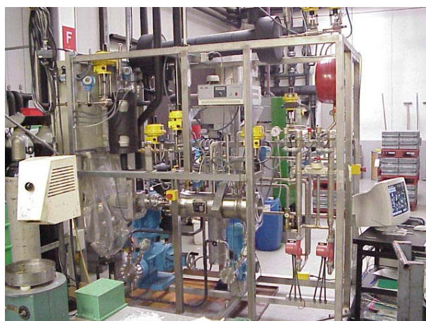
Clamp-On Agitation of the Liquid, Supercritical CO 2 Reactor (300 Bar applications, 25 mm wall thickness)
